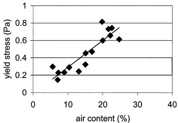
Fig. 8—Yield stress of paste versus air content at  $w/c$  0.30 for Admixture A dispersed with high-range water-reducing admixture (fitted to linear function).
