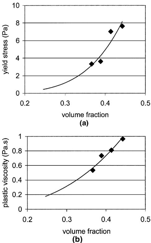
Fig. 12—Rheological parameters of paste versus volume fraction of solids for data at zero air extrapolated from Fig. 4 and 5, showing: (a) yield stress; and (b) plastic viscosity (both fitted to power functions).
