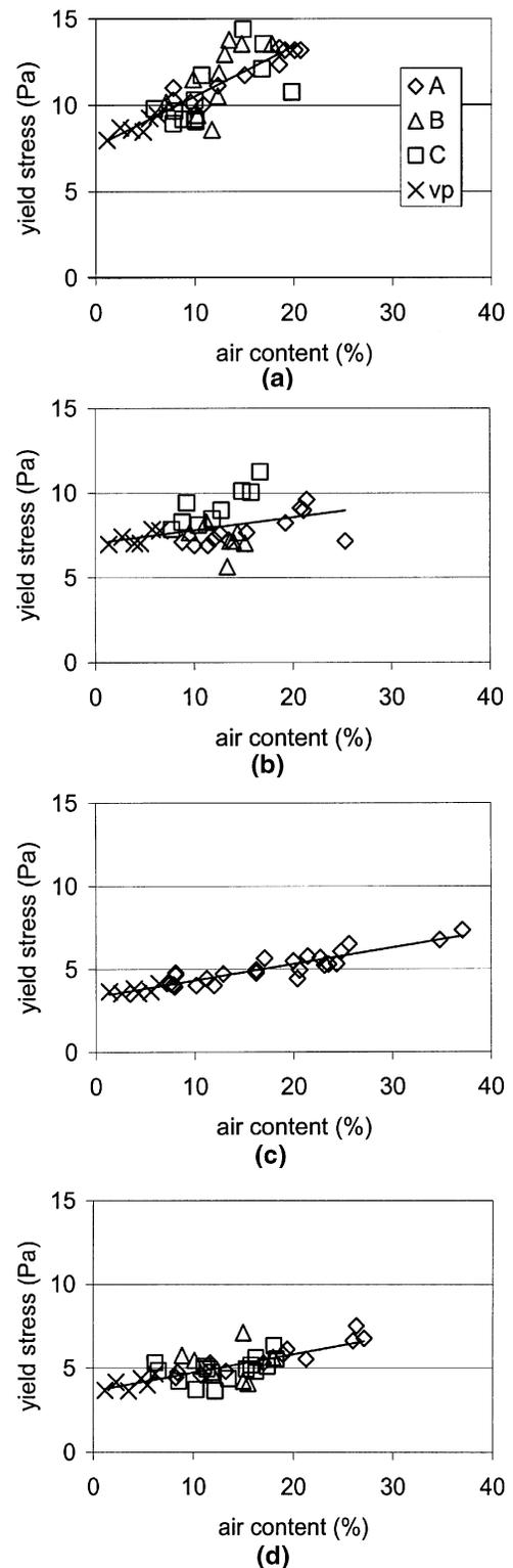
Fig. 5—Yield stress of paste versus air content at: (a) *w/c* 0.40; (b) *w/c* 0.45; (c) *w/c* 0.50; and (d) *w/c* 0.55 for Admixtures A, B, and C and vacuum-processed (vp) paste (fitted with linear functions).
