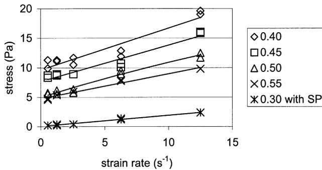
Fig. 4—Flow curves (stress versus strain rate) of pastes at various *w/c* levels with no air-entraining admixture, including paste at *w/c* 0.30 dispersed with high-range water-reducing admixture (fitted with linear functions).
