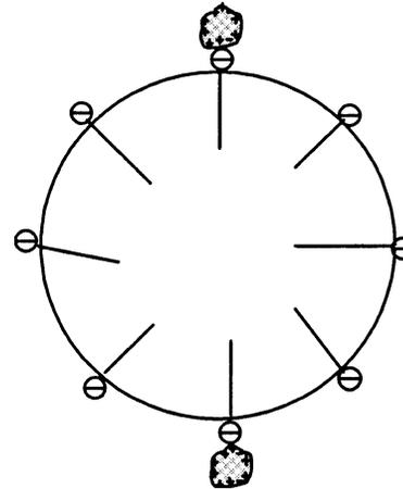
Fig. 14—Schematic diagram of bubble bridging cement particles.
