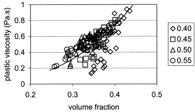
Fig. 13—Plastic viscosity of paste versus volume fraction of solids for all data with power function at zero air from Fig. 12(b).
