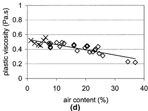
Fig. 6—Plastic viscosity of paste versus air content at: (a) w/c 0.40; (b) w/c 0.45; (c) w/c 0.50; and (d) w/c 0.55 for Admixtures A, B, and C and vacuum-processed (vp) paste (fitted with linear functions).
