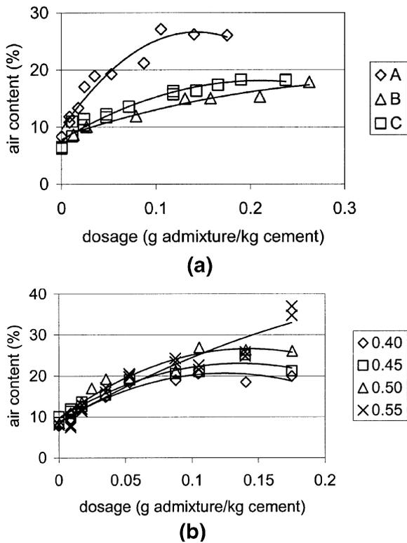
Fig. 3—Air content of paste versus dosage of air-entraining agent: (a) at  $w/c$  0.50 using various air-entraining agents; and (b) at various  $w/c$  levels using Admixture A (fitted with polynomial functions).
