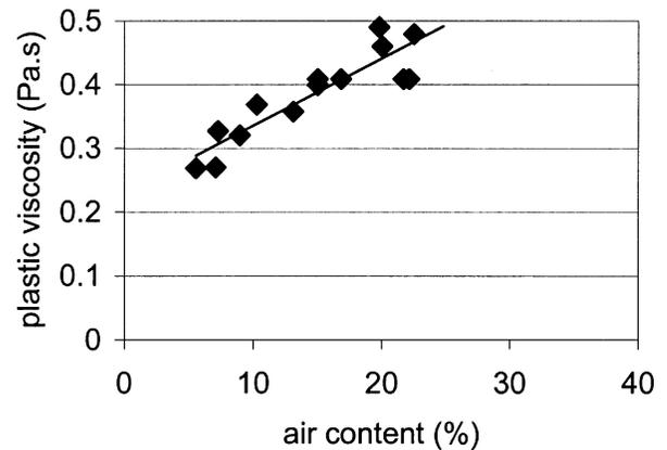
Fig. 9—Plastic viscosity of paste versus air content at  $w/c$  0.30 for Admixture A dispersed with high-range water-reducing admixture (fitted to linear function).
