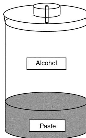
Fig. 1—Density bottle used to measure air content of fresh paste.
