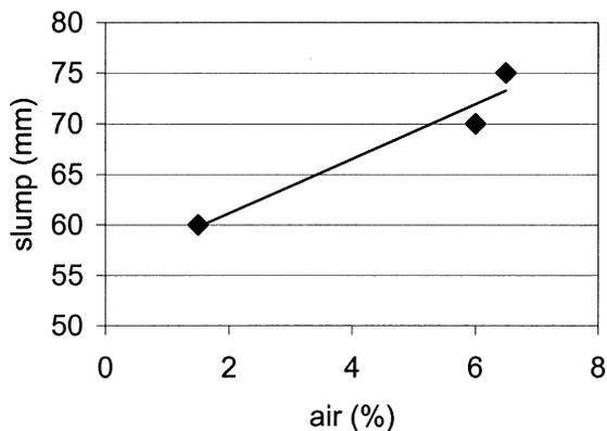
Fig. 15—Slump of concrete versus air content.
