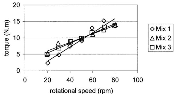
Fig. 10—Flow curves (torque versus rotational speed) of concretes in Table 3.
