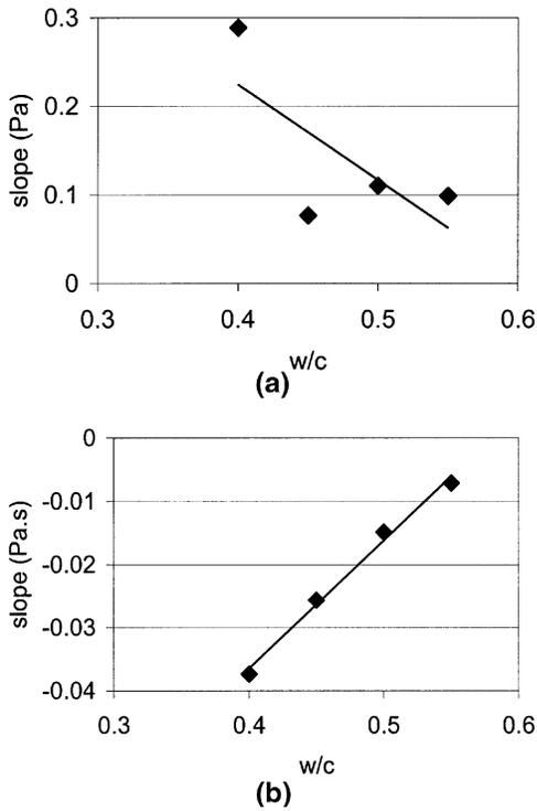
Fig. 11—Slope relating paste rheology to paste air content versus  $w/c$ , showing: (a) slope relating yield stress to air content (from Fig. 5); and (b) slope relating plastic viscosity to air content (from Fig. 6).
