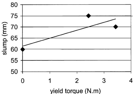
Fig. 16—Slump of concrete versus yield torque.
