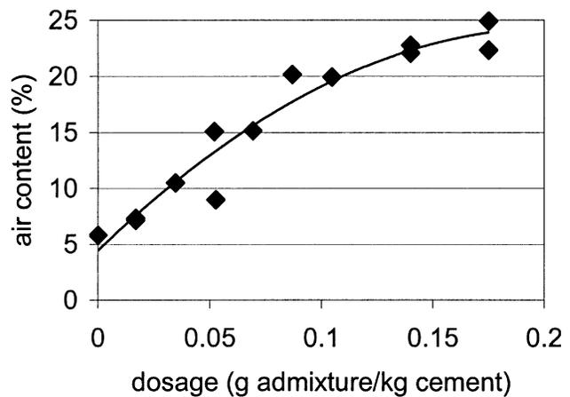
Fig. 7—Air content of paste versus dosage of air-entraining agent at w/c 0.30 using Admixture A dispersed with high-range water-reducing admixture (fitted to polynomial function).
